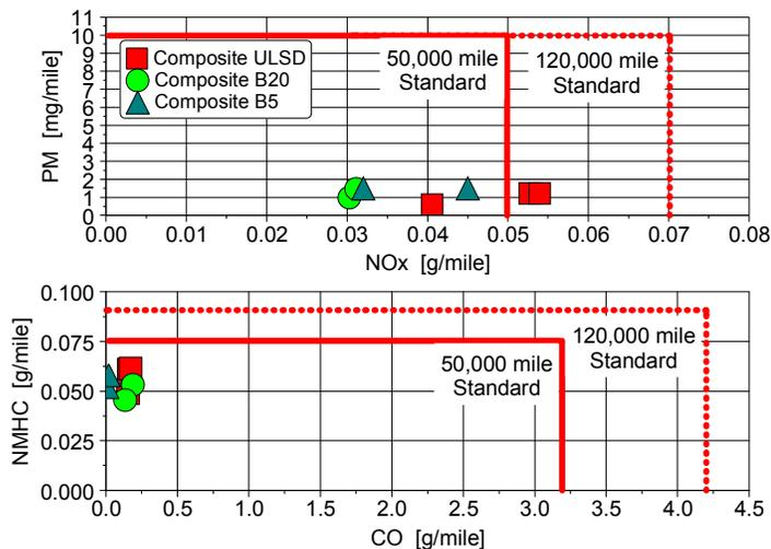
Figure 18: Composite emissions comparison with NAC system
