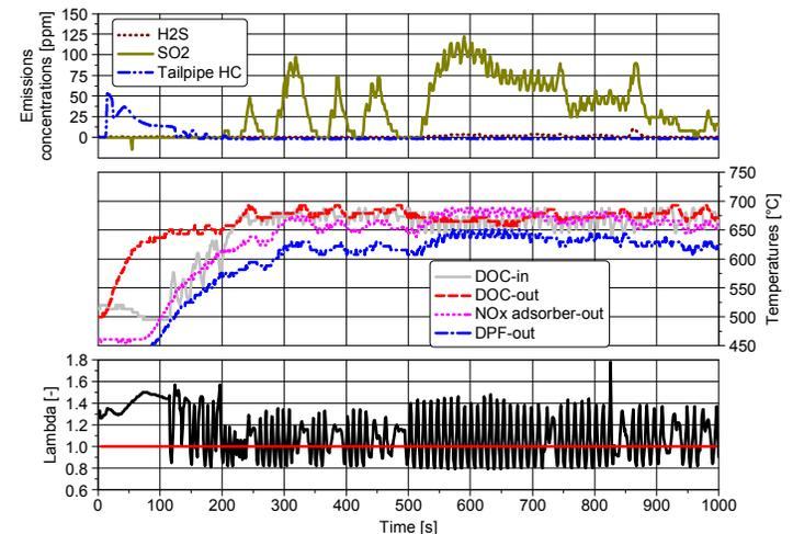
Figure 14: Desulfurization under steady-state conditions with B20 (engine test cell)
