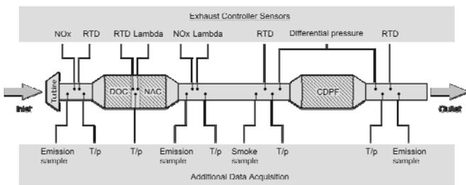
Figure 2: NO<sub>x</sub> adsorber catalyst/DPF emission control system
