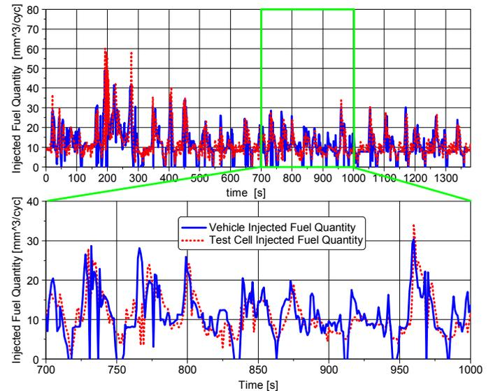
Figure 6: Fuel quantity comparison test cell and vehicle
