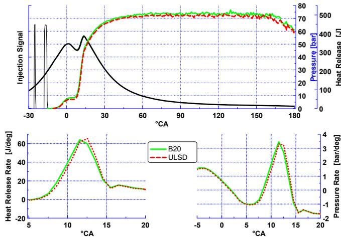
Figure 21: Combustion analysis 1500 rpm, 15 mm<sup>3</sup>/cycle
