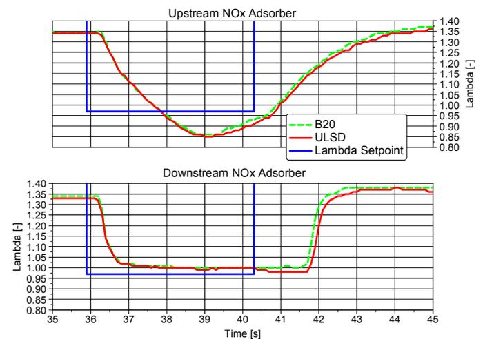
Figure 12: Biodiesel effects on lambda during lean-rich modulation (engine test cell)
