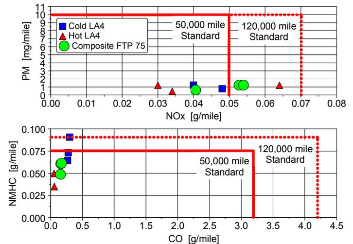
Figure 17: ULSD emission results with NAC system
