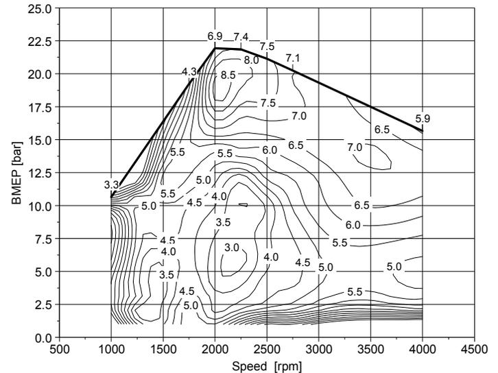
Figure 1: Engine-out NO<sub>x</sub> [g/kWh]
