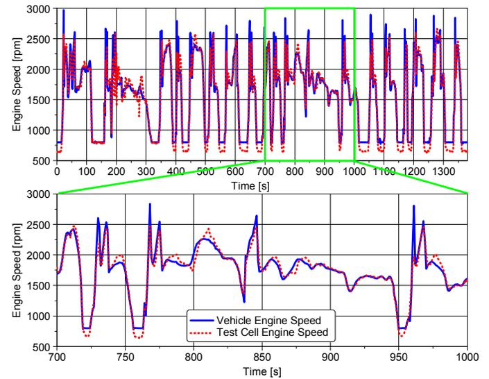
Figure 5: Engine speed comparison test cell and vehicle
